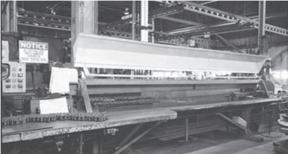
All Cast and Cast Combination chains are 100% inspected and proof tested to ensure that no poorly molded links leave the factory.
